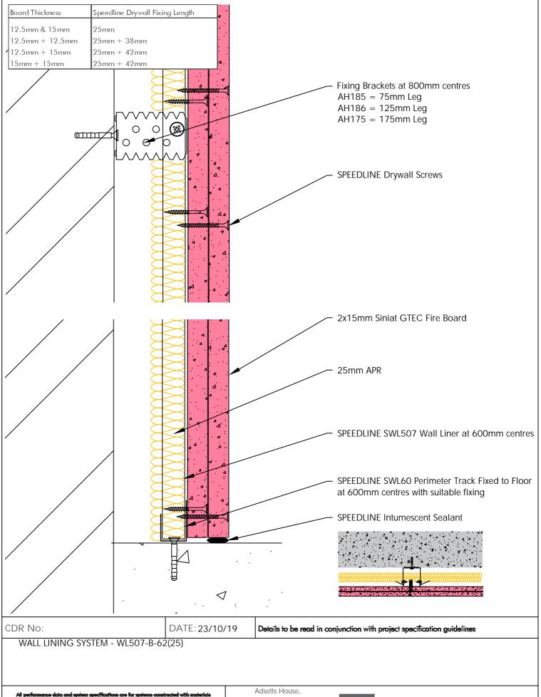
All performance data and system specifications are for systems constructed with materials & components as shown. The inclusion or substitution of any other manufacturers materials or components could invalidate test data and system performance and permission must be given in writing by SIG FLC.
